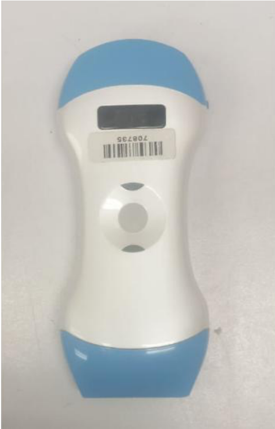
Figure 1. Image of the handheld Ultrasound that was used for the pleural procedures. It connects wirelessly to a smartphone or tablet.
